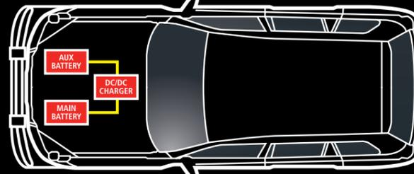
A sophisticated dual battery charger engineered for in-vehicle or under bonnet installation on vehicles fitted with traditional or smart alternators
